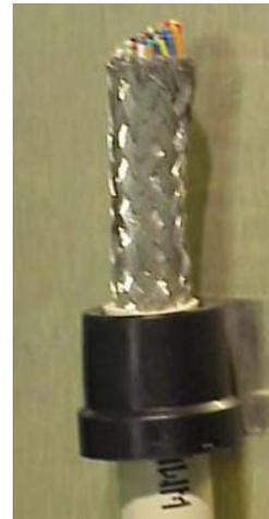
Figure AH-6. Metal Braid Hydraulic Lines, corrugated gas appliance line and braided shielded cable all work well for EMC shielding of 5-wire sensor connections.
